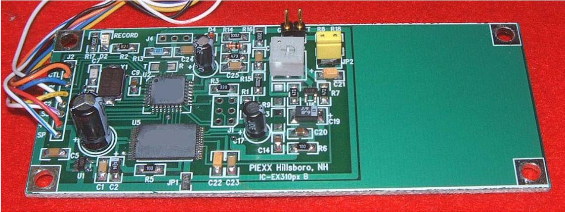
The PIEXX IC-EX310px is a physical and electrical replacement for the original ICOM IC-EX310 speech synthesizer.
