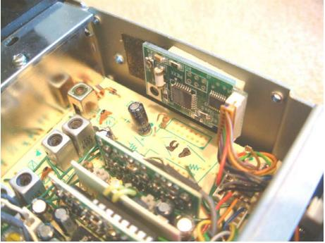
FTS-12px installed in radio. Note the cut 27K resistor.5. Complete the installation by reinstalling the FT-211RHs bottom cover.
