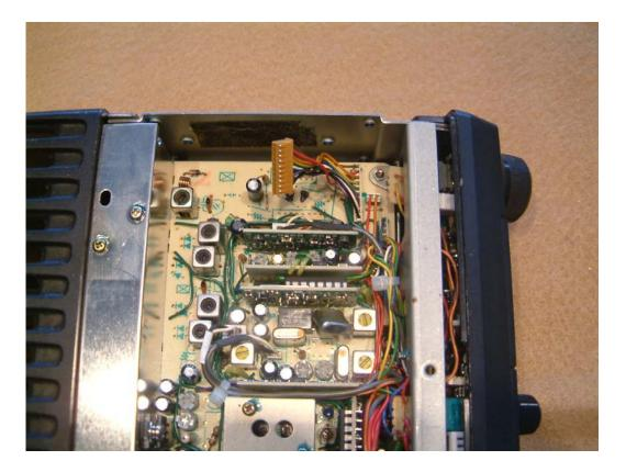
3. Use double-sided adhesive tape to attach the FTS-12px to the side chassis of the transceiver. The FT-211RH came equipped with a piece of double stick tape in the appropriate spot ready for FTS-12 installation.
