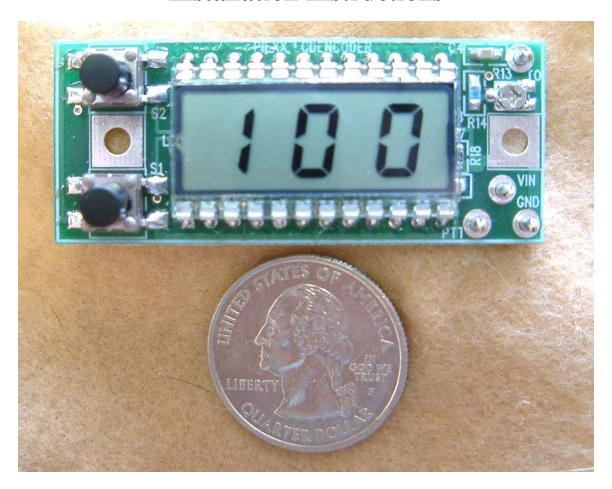
The PIEXX LCDENCODER is a general purpose CTCSS tone encoder board that has a direct reading LCD display to show the current operating tone frequency. The LCDENCODER is easy to install as it requires only a 5-16VDC power source and a connection between the Tone Output and your transceivers audio in circuitry. Optionally you can connect the PTT line to enable / disable the tone output except when in transmit mode.
