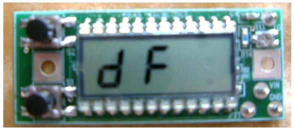
dF stands for display Flip. If the dF is upside down, flip the board over so it reads correctly. To flip the display, press the top button. Please be aware that not only is the display flipped, but which button is top is also flipped, so if the dF display is upside down you will need to press the bottom button to get it right side up again. That is, you make the selection with the top button when the display is showing
