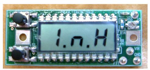
InH - CTCSS tone generation when the PTT input line is floating or has a positive value
