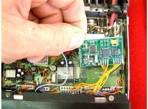
3. Use double-sided adhesive tape to attach the UT-29px to the PC board in your radio in the location marked 'OPTION UNIT'.
