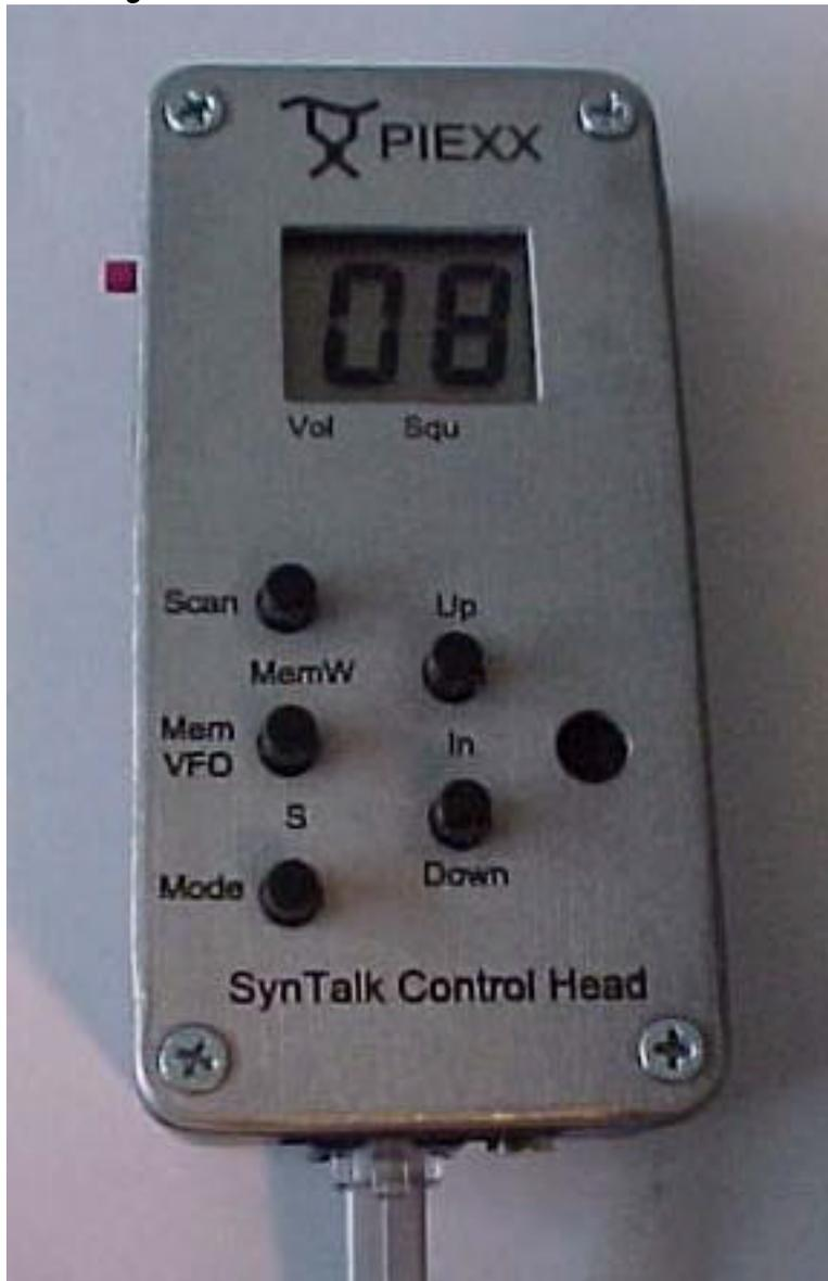
The Syntalk Control Head / Microphone is intended to allow operation of the Syntalk converted Syntor transceiver without the use of a dedicated computer. Although the control head is primarily intended for channelized operation, it is capable of the following operations:
