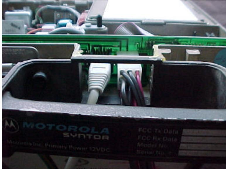
22. Connect the 8 pin RJ-45 cable to its mating receptacle from the front of the transceiver. The other end of this RJ-45 cable will connect to the SYNMIC breakout board in the modular jack marked 'SYNTOR'
