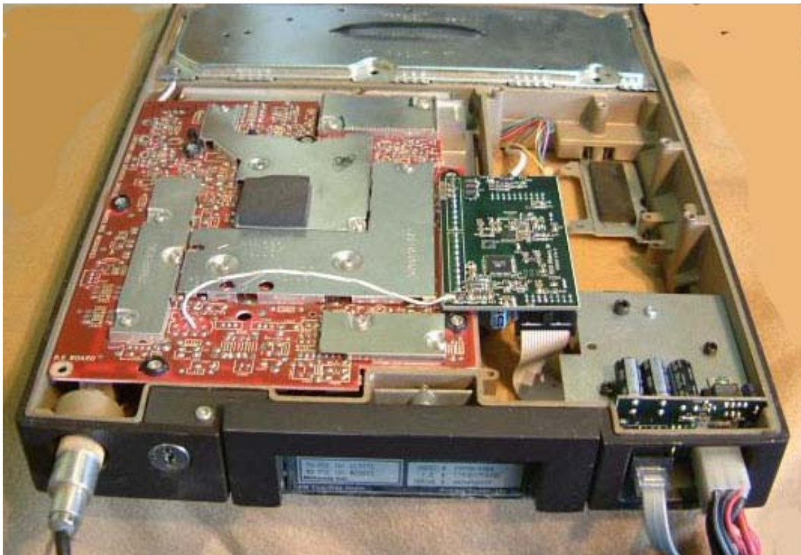
Syntor X Transceiver with PIEXX SynControl Installed
