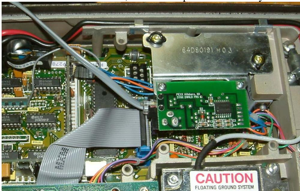
5. The revision C serial interface adapter has mounting holes that will allow it to be permanently installed in the radio. If you plan on leaving the serial interface adapter in the radio, you will need to make an exit hole in the case for the serial cable.
