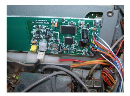
4. Install the 8-pin cable, coming from the IC-EX310px board, onto the J12 connector on the IC-751 logic board.
