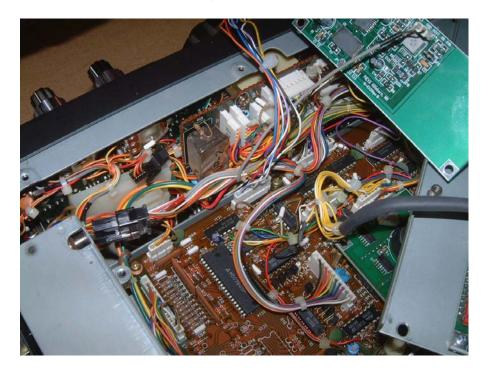
4. Locate the 2 pin cable, coming from the front of the radio, whose connector is marked 25. Install this plug on the 2-pin header marked J3 on the IC-EX310px board. Make sure to orient the connector so that the shield part of the cable attaches to the pin marked GND. When properly oriented, the 25 printed on the cable will be closes to the edge of the board..
