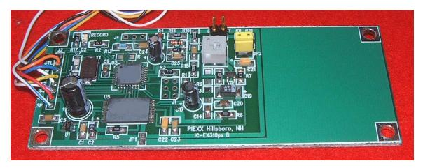
The PIEXX IC-EX310px is a physical and electrical replacement for the original ICOM IC-EX310 speech synthesizer.
