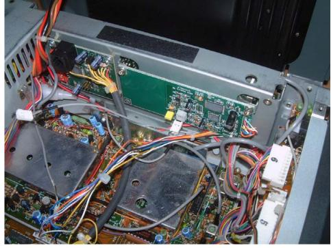
3. Locate the 2 pin cable, coming from the right rear of the radio, whose connector is marked 31. Install this plug on the 2-pin header marked J3 on the IC-EX310px board. Make sure to orient the connector so that the shield part of the cable attaches to the pin marked GND. When properly oriented, the 31 printed on the cable will not be visible.
