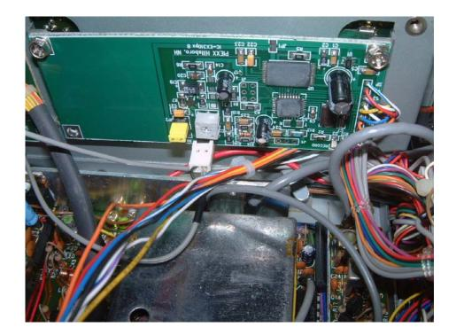
4. Install the 8 pin cable, coming from the IC-EX310px board, onto the J12 connector on the IC-751A logic board.
