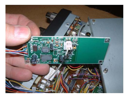
5. Replace the Logic board cover plate, then mount the IC-EX310px board on the 4 standoffs located in the center of the mounting plate.
