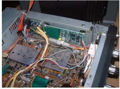
3. Locate the 2 pin cable, coming from the right rear of the radio, whose connector is marked 34. Install this plug on the 2-pin header marked J3 on the IC-EX310px board. Make sure to orient the connector so that the shield part of the cable attaches to the pin marked GND. When properly oriented, the 34 printed on the cable will not be visible.
