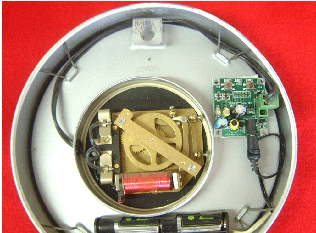
IMP-22 Inside Gents Clock. Since the Gents Mechanism is Bipolar, clock leads are in the top two terminals of the IMP-2 terminal Strip.
