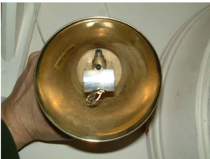
A 24VDC Solenoid mounted inside of a 4" Bell for Hour Strike
