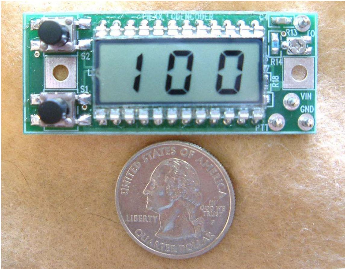
The PIEXX LCDENCODER is a general purpose CTCSS tone encoder board that has a direct reading LCD display to show the current operating tone frequency. The LCDENCODER is easy to install as it requires only a 5-16VDC power source and a connection between the Tone Output and your transceivers audio in circuitry. Optionally you can connect the PTT line to enable / disable the tone output except when in transmit mode.
