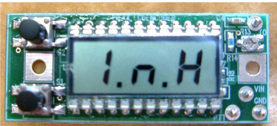
InH - CTCSS tone generation when the PTT input line is floating or has a positive value
