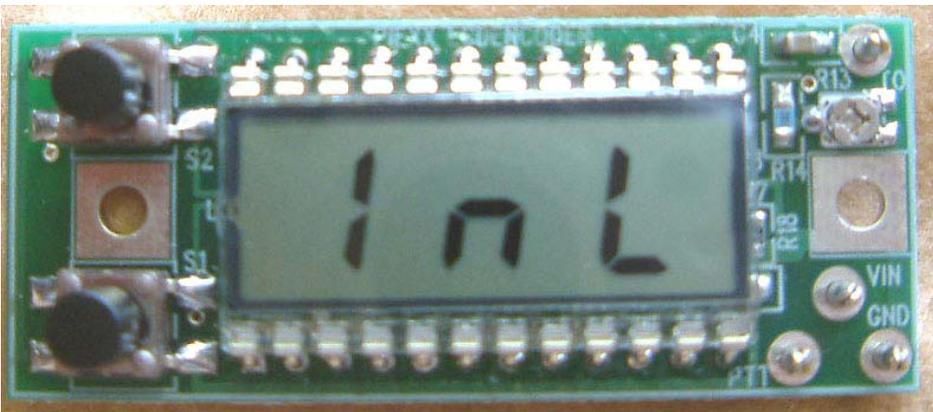
InL – CTCSS tone generation when the PTT input line is pulled to a ground level.
