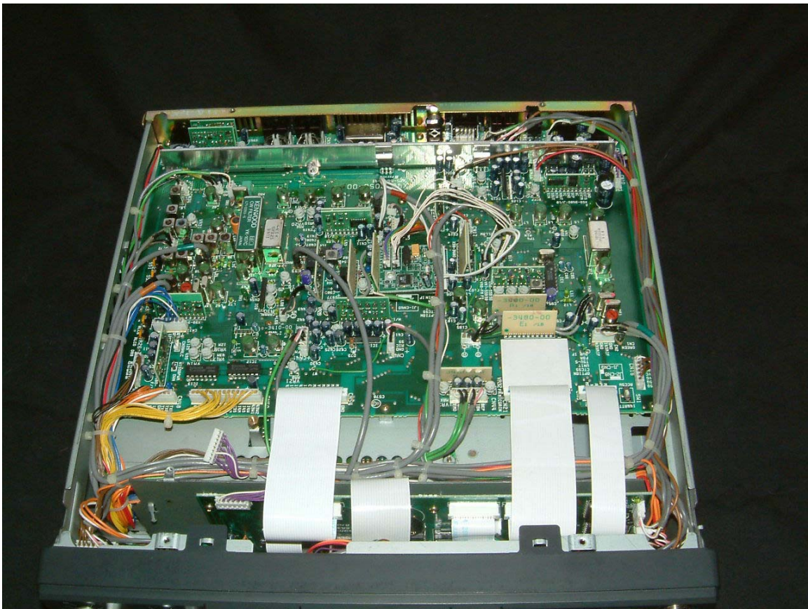
TSU5Dpx installed in TS-790A Transceiver
