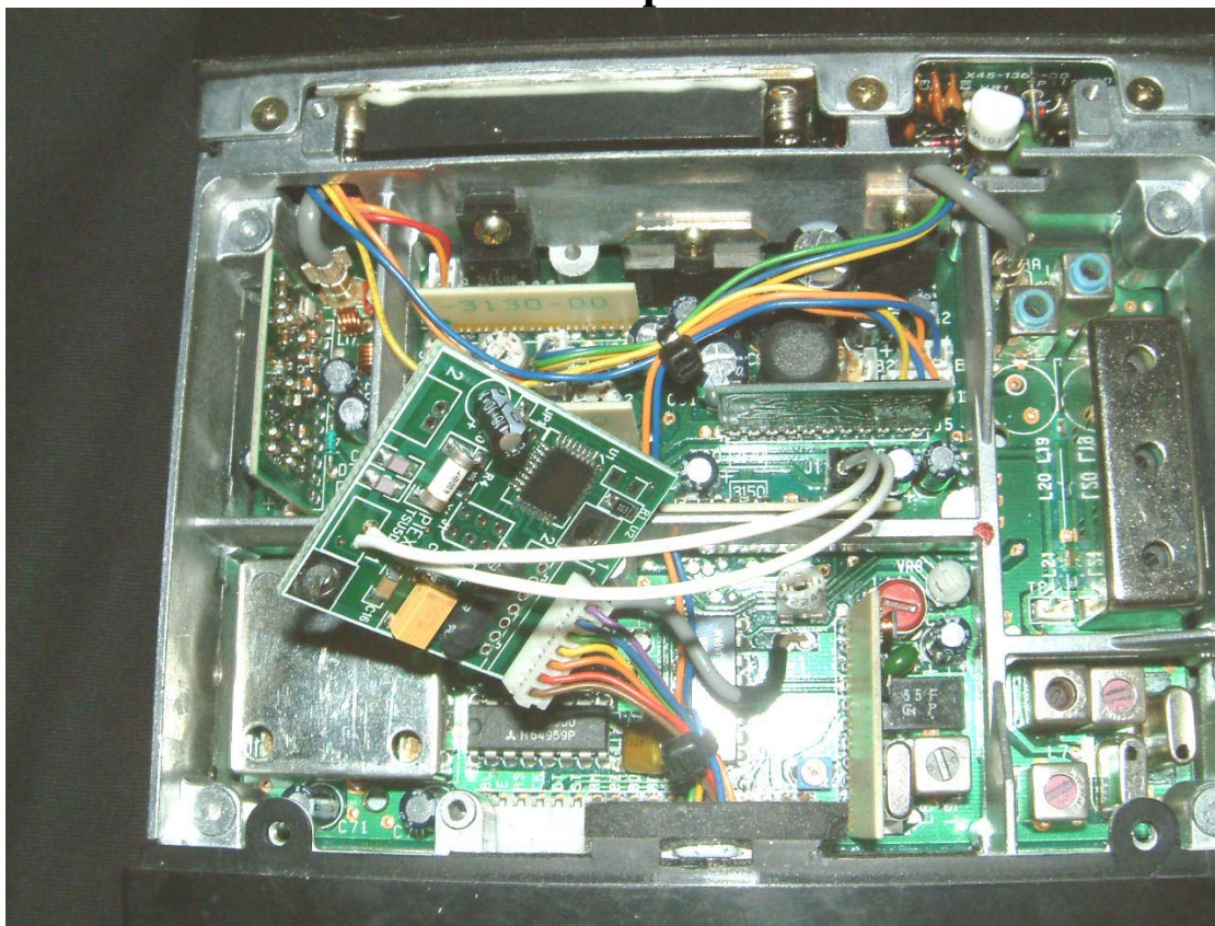
TSU-5px Installed in the TM-221A. Note 7 pin Connector Orientation.
