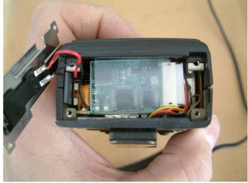
7. Complete the installation by reinstalling the battery mounting track and battery pack.
